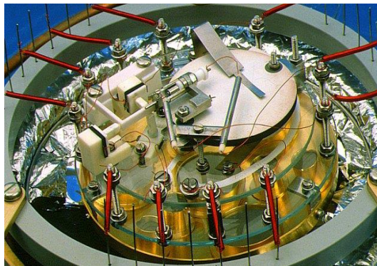
Exact copy of first Scanning Tunneling Microscope of Binnig and Rohrer (original has not preserved).
